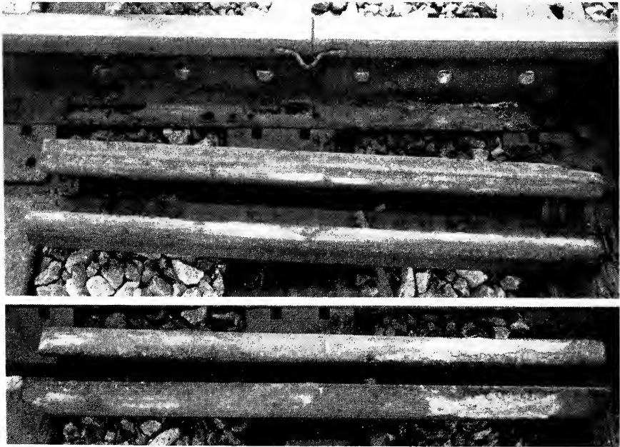
Fig. 15. West Rail Section 3, Spray Coat of Texaco No. 941 after One Year of Service
